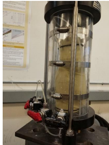
(b) Shear failure
